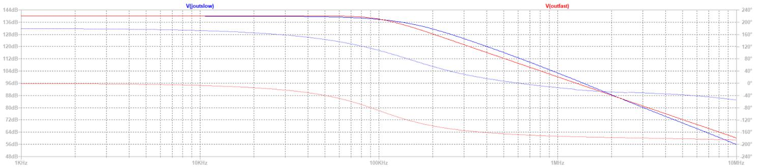
Figure 6: The red traces show the current gain of the simple TIA with a “fast” op amp (AD8065, 145MHz GBP) while the blue traces show the current gain of the TIA with a JFET and a “slow” op amp (ADA4610, 15.4MHz GBP).  $C_{pd} = 100\text{pF}$  in both cases.
