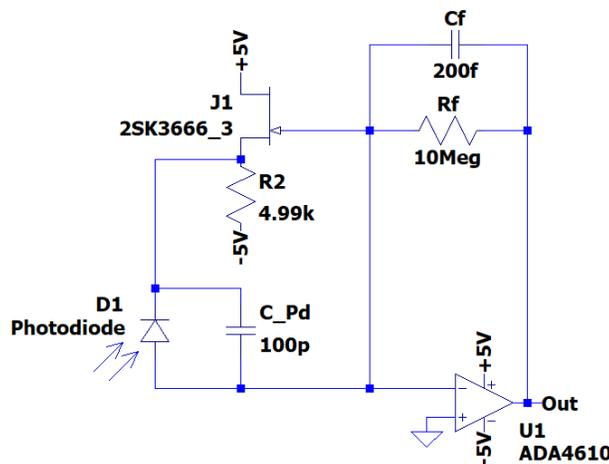
Figure 4: High-Gain TIA with JFET on Input (explicitly showing photodiode capacitance). The ADA4610 has a 15.4-MHz GBP.
