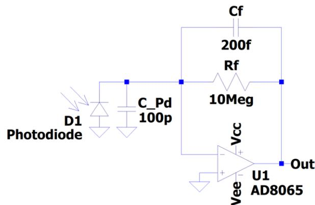
*Figure 1: Conventional Simple High-Gain TIA (explicitly showing photodiode capacitance) The op amp has a 145MHz GBP.*
