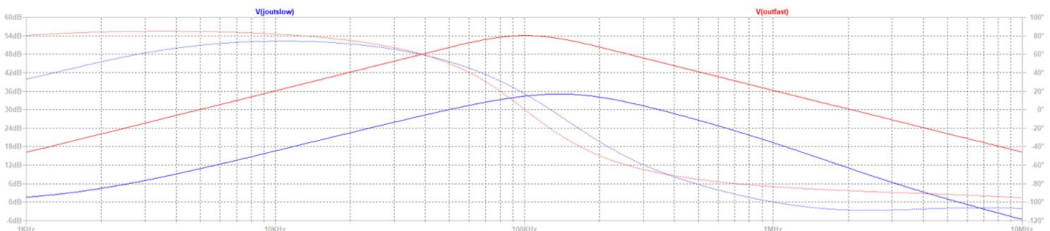
Figure 5: The red traces show the voltage gain of the simple TIA with a "fast" op amp (AD8065, 145MHz GBP) while the blue traces show the voltage gain of the TIA with a JFET and a "slow" op amp (ADA4610, 15.4MHz GBP).  $C_{Pd} = 100\text{pF}$  in both cases.
